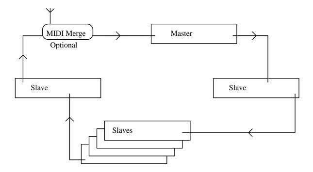
Any DN3600 in the loop can be designated as the Master by entering the Slaves sub menu (press **Utilities, More..., Slaves**). The other DN3600 and DN3601 units in the loop will automatically configure themselves as slaves, with the first being number 1, the second being number 2 and so on. A maximum of 64 slaves may be connected in this way (65 units including the Master).
